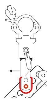
Note: For higher negative / positive vertical frame angles, it's necessary to place the Adapter into the right direction.
