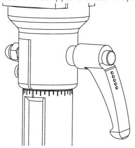
2. Rotate the rotating module of Vario Clamp to the desired position. To adjust the angle of the rotation, use the scale and rotate to the left or to the right (the scale shows the angle, one division corresponds to 10°).
