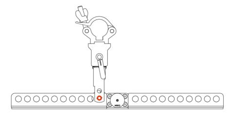
Example shows the Vario Clamp combined with FRV-APS. Pin Position 2.
