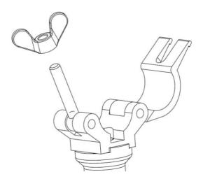
▲ When Half Coupler is in its open position, Vario Clamp can be lifted and placed on the metal farm intended for mounting the construction.
