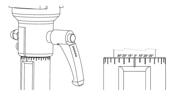
3. When aligned as intended, pull the adjustable hand lever to fix the rotating module.
