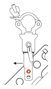
Note: For higher negative / positive vertical frame angles, it's necessary to place the Adapter into the right direction.
