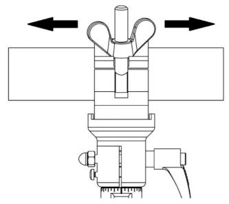
A Note: While adjusting the horizontal position of the Vario Clamp hold the Vario Clamp the entire time. Because Vario Clamp is heavily loaded at the same time the wingnut is not fully tighten there is a hazard of falling of heavy loads from the metal farm
