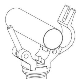
Step 3. Close and lock the two parts of the Half Coupler enclosing the pipe, respectively the metal farm.
