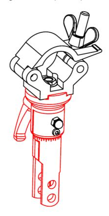
1. To loosen the rotating module of Vario Clamp push the button and pull the adjustable hand lever.
